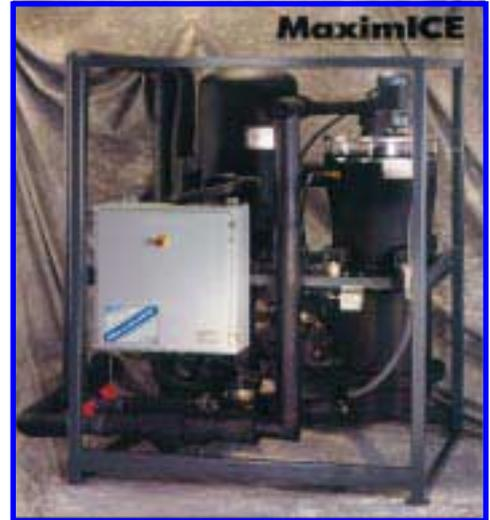
At 20-25% ice concentration, Slurry-ICE flows like conventional chilled water whilst providing 5 times the cooling capacity. At higher ice concentrations, it still demonstrates pumpable characteristics.
